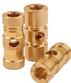
The design of the Z-bearing is popular on the smaller turbos because it simplifies the assembly by incorporating the thrust bearing faces onto the ends of the journal bearing. The design means that there are fewer parts, and hence less room for accumulated tolerance and balancing errors. The detail of the oil ramping on the thrust face also
